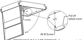
**REMOVING BALLAST SCREWS:** Remove screw holding the ballast cover to fixture.
