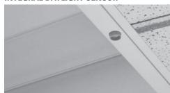
**APPLICATION:** Daylight sensor is a turn key solution for lighting control. Integral sensor is wired to the 0-10 volt dimming ballast at the factory. No additional wiring is required by the contractor.
