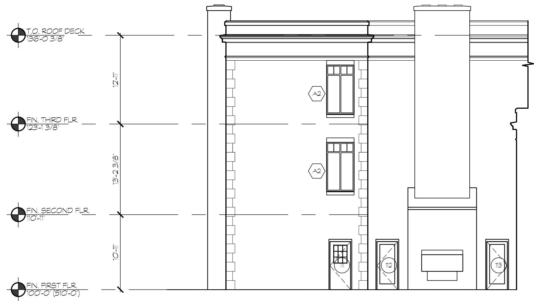
PART. SOUTH ELEVATION - NEW WORK 1/8" = 1'-0" 3 A3.2
